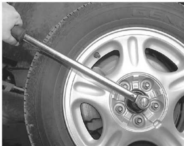
Tighten the wheel lug nuts using a torque wrench
