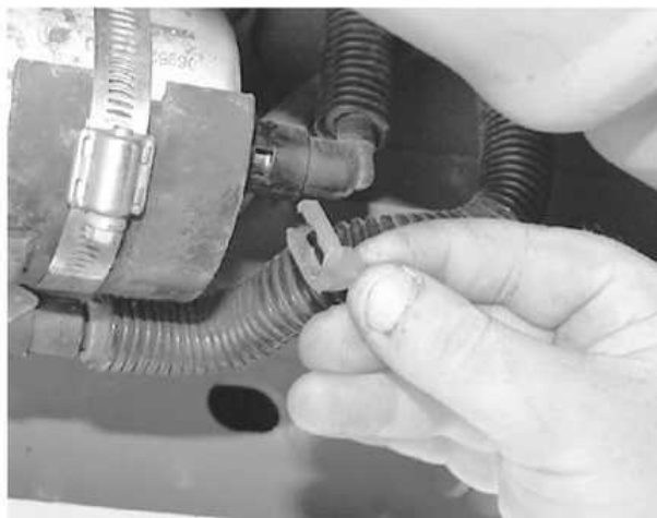
Remove the clips from the push connect fittings.
