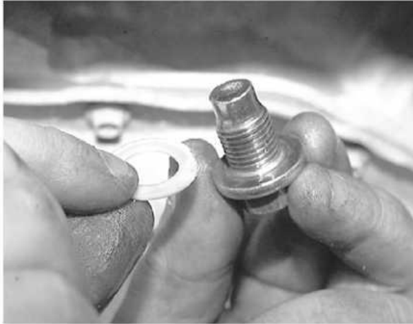
Inspect the threads on the drain plug as well as the gasket and replace either if necessary
