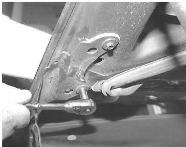
Remove the hood hinge-to-hood retaining bolts
