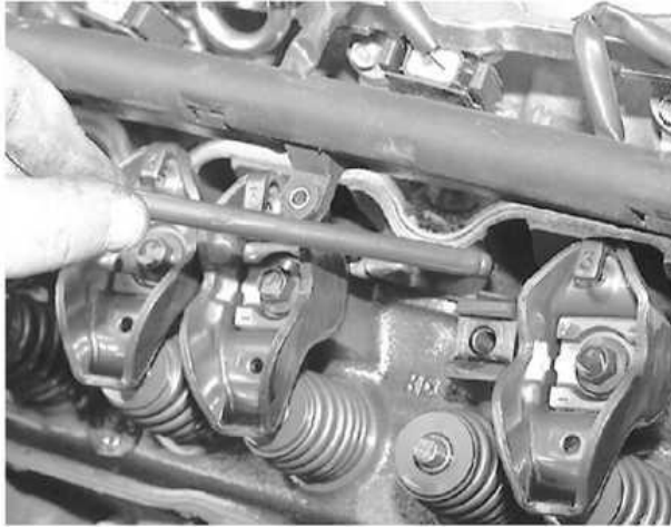
Remove the push rods from the engine if necessary.
