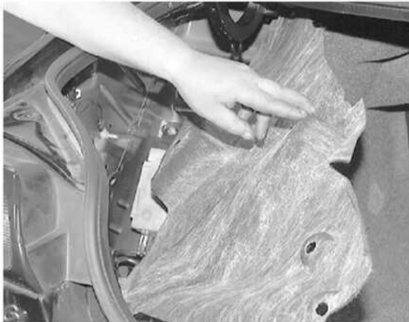
Remove the trim to access the rear chassis unit
