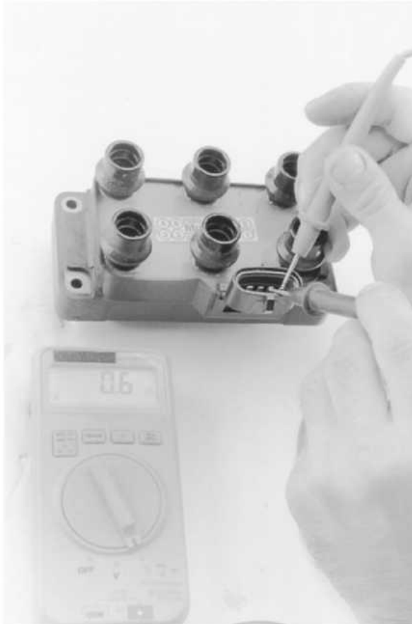
Testing the coil primary resistance using a multimeter
