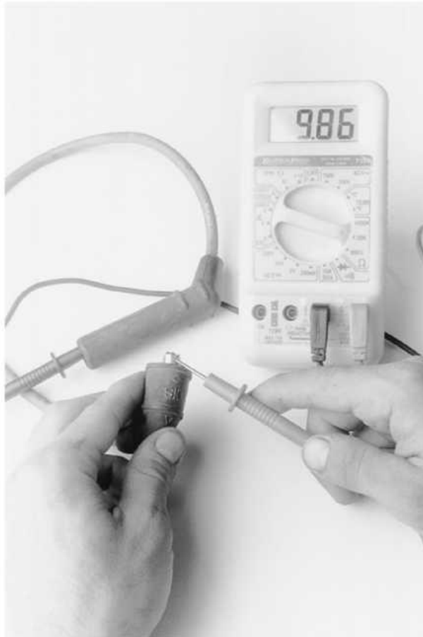
Spark plug wires can be checked for excessive resistance using an ohmmeter
