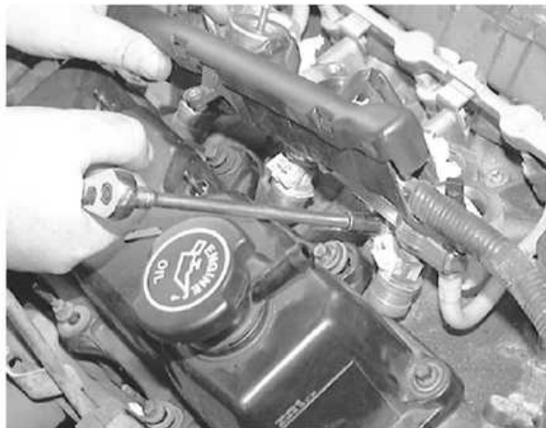
Remove the fuel rail retaining bolts from the front and the...
