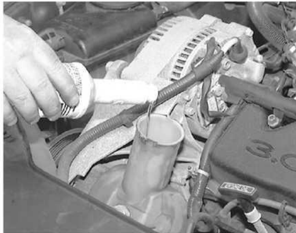
Carefully pour the power steering fluid directly into the reservoir
