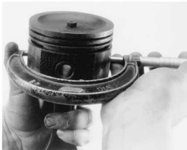
Measure the piston's outer diameter, perpendicular to the wrist pin, with a micrometer
