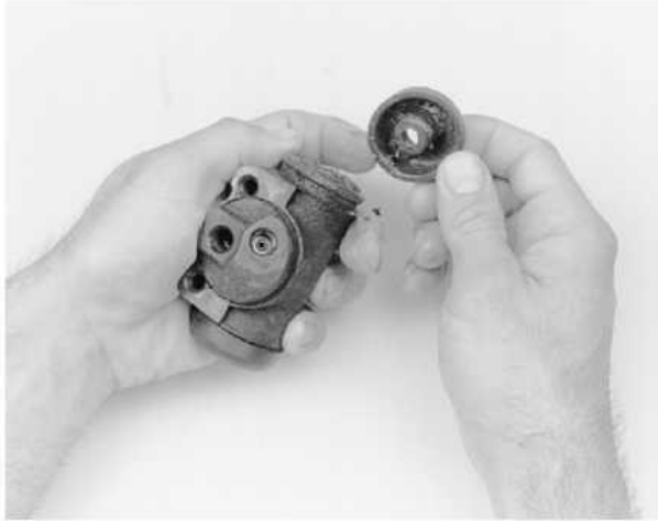
Remove the outer boots from the wheel cylinder
