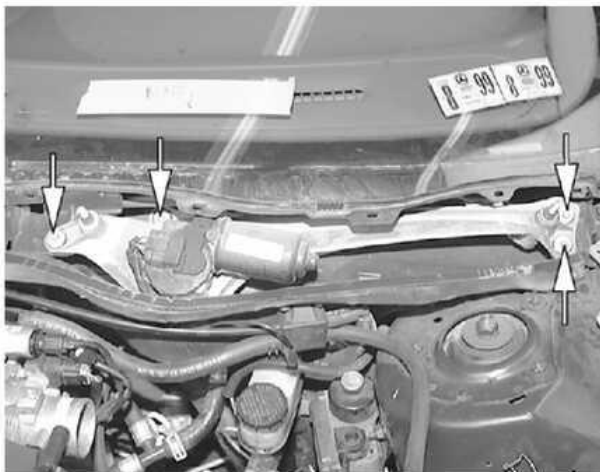
Remove the four wiper module retaining bolts and...
