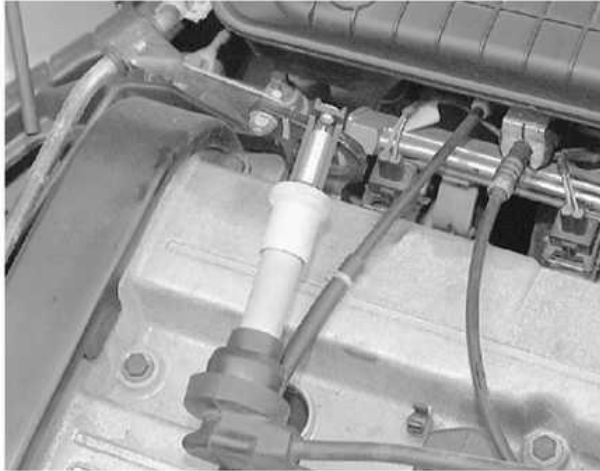
Attach the clip to ground and crank the engine to check for spark
