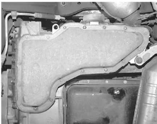
The transaxle fluid pan is retained by 17 bolts
