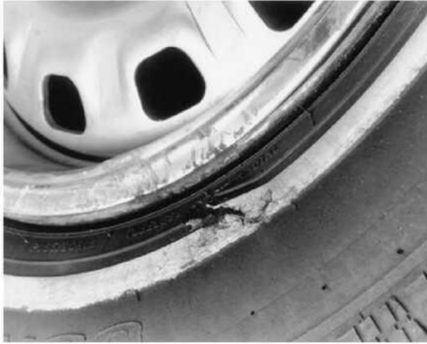
Tires with deep cuts, or cuts which bulge, should be replaced immediately
