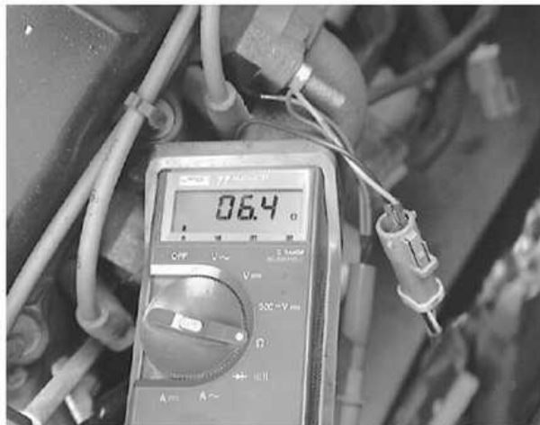
The voltage of the HO 2 S should be between 0.1 and 1.0 volts DC with the engine running.
