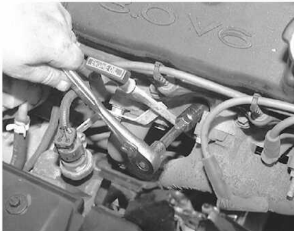
Use a spark plug socket and the proper drive tools to remove the plug from the engine. The spark plug on the 3.0L OHV engine requires a 5/8 socket
