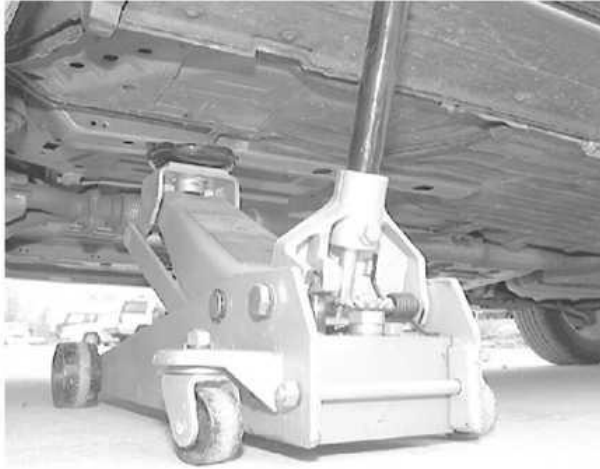
Place the jack under the frame rails to lift the front of the vehicle
