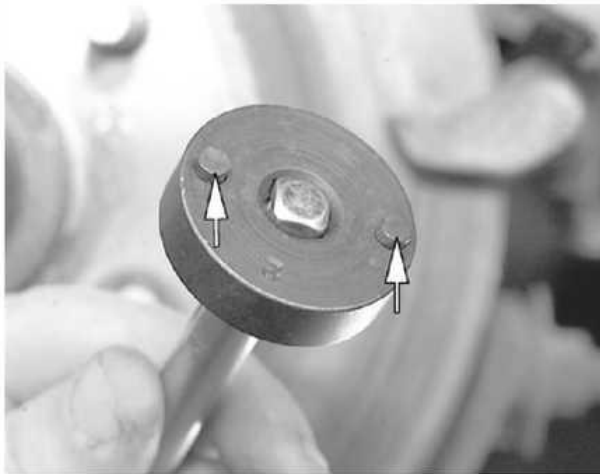
The caliper piston shown is used to rotate the piston and compress it. Align the small pins with...
