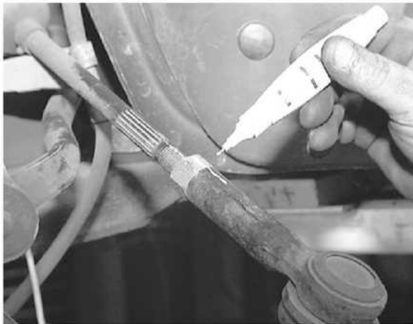
Mark the outer tie rod jam nut on one side with a reference line for installation.
