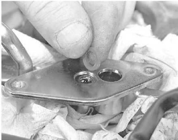
... the rail with new O-rings
