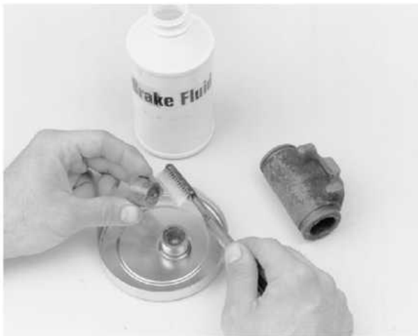
Use brake fluid and a soft brush to clean the pistons...
