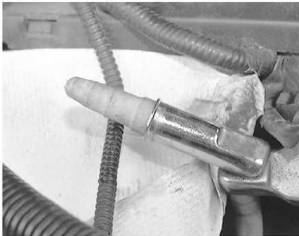
the inlet on the fuel rail to prevent contamination of the fuel system
