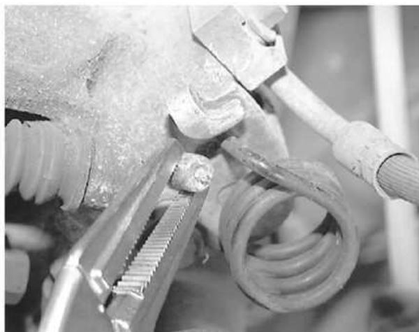
... remove the cable from the caliper
