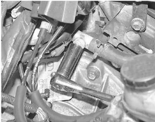
Remove the temperature gauge sending unit using a suitable tool
