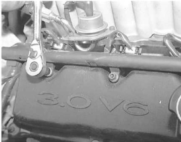
Remove the fuel injector harness retaining nuts and...
