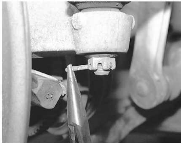
Remove the cotter pin from the tie rod end and...
