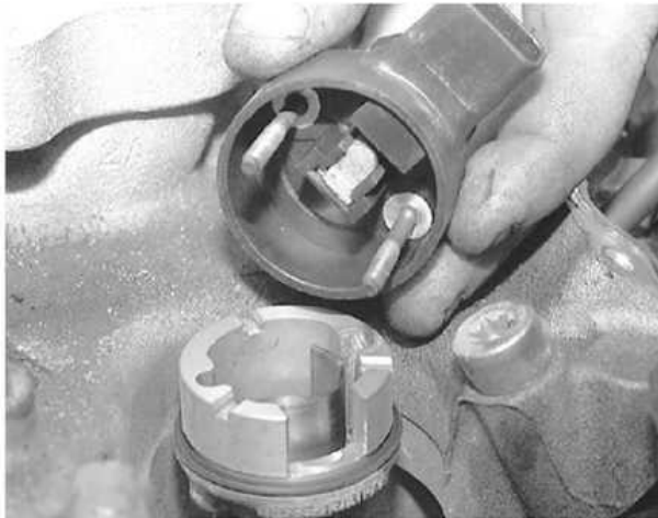
Remove the two retaining screws and remove the sensor from the housing
