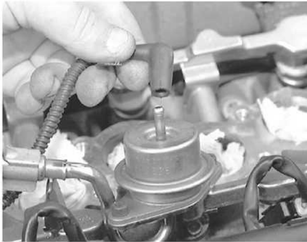
Disconnect the vacuum hose from the pressure regulator
