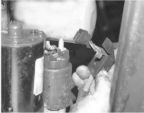
... remove the battery cable from the starter
