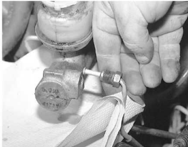
... disconnect the brake lines from the master cylinder
