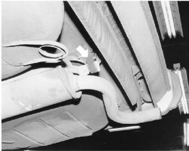
Check for overstretched or torn exhaust hangers
