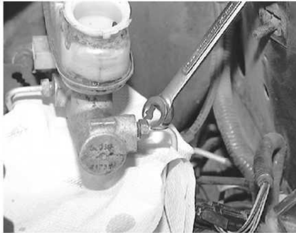
Use a flare nut wrench to...
