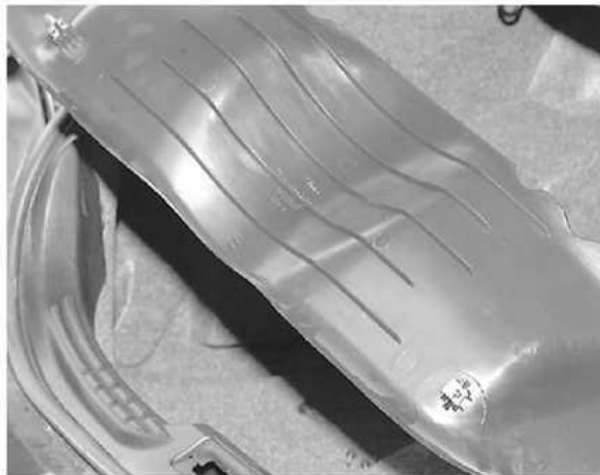
Remove the trim from the underside of the trunklid
