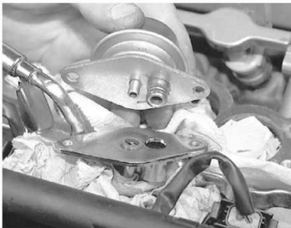
... remove the regulator from the injector rail
