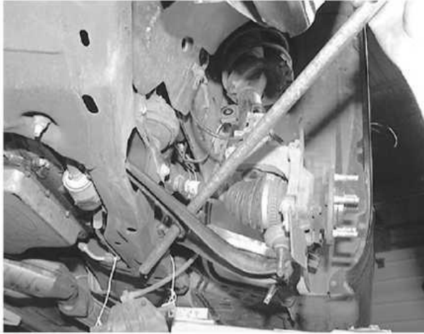
Using a pry bar or other suitable tool, remove the lower ball joint from the knuckle.
