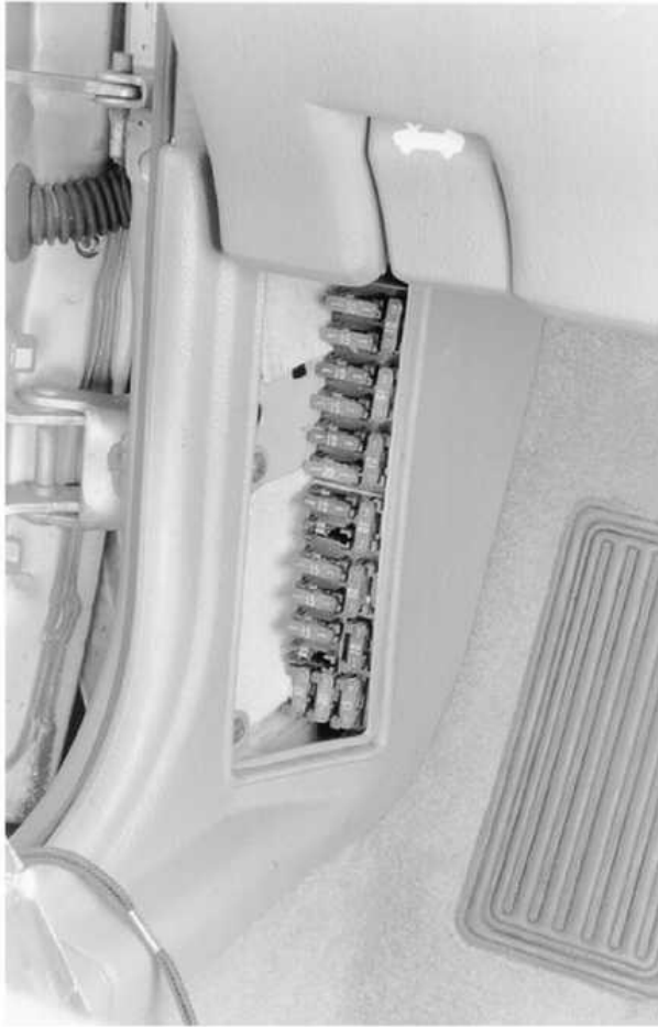
Most vehicles use one or more fuse panels. This one is located on the driver's side kick panel
