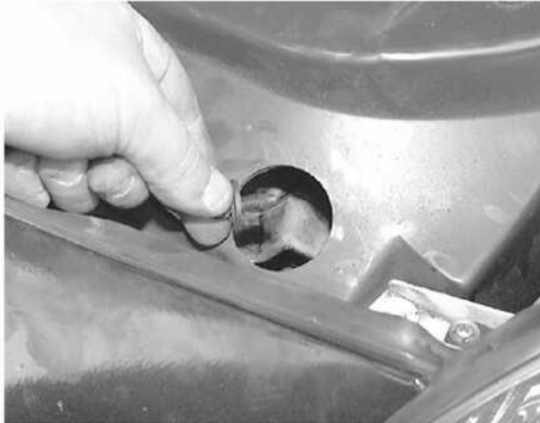
The upper radiator retaining screws are accessible through a hole, remove them from the radiator
