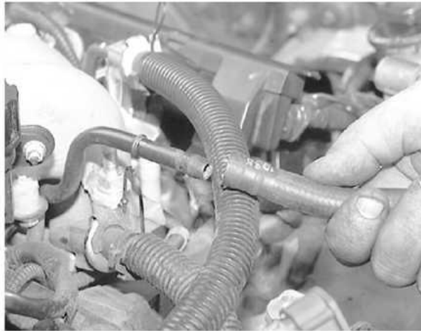
... remove the hose from the tube
