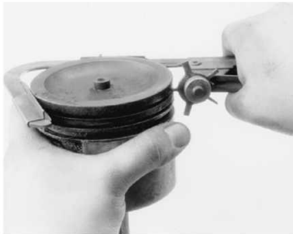
Clean the piston ring grooves using a ring groove cleaner tool, or...
