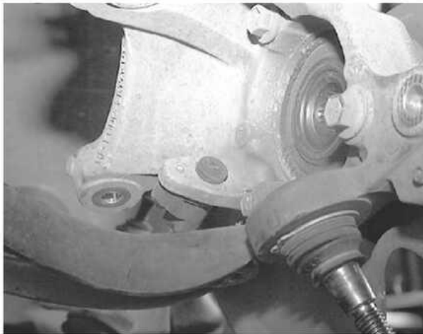
Separate the ball joint from the lower control arm
