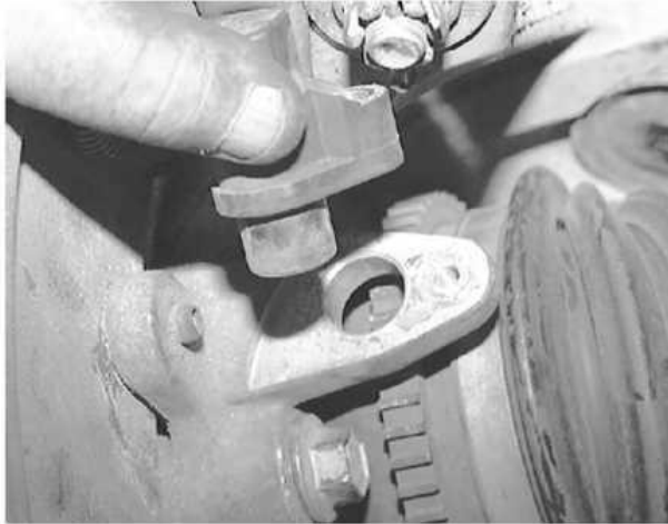
... remove the sensor from the front steering knuckle
