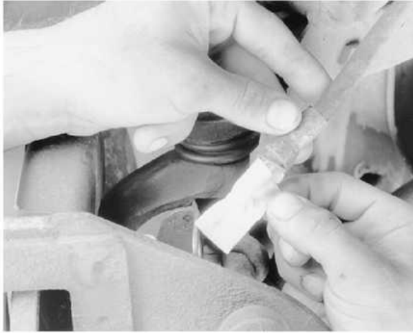
Tape or plug the line to prevent contamination
