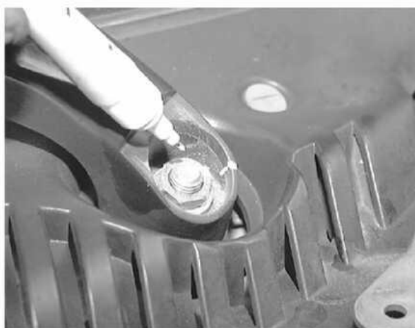
Matchmark the wiper arm-to-pivot
