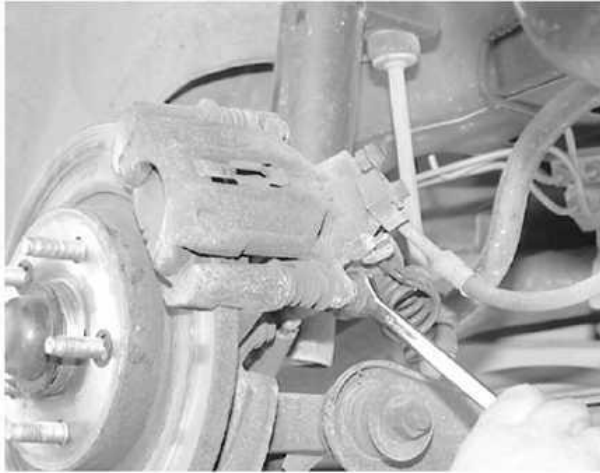
... lower caliper locating pins. The lower locating pin must be removed using a wrench to clear the parking brake actuator spring
