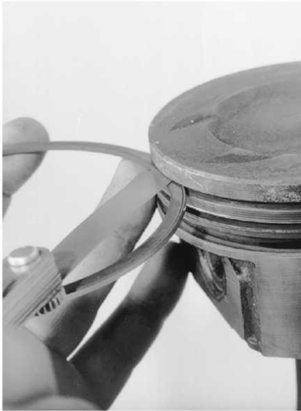
Checking the piston ring-to-ring groove side clearance using the ring and a feeler gauge
