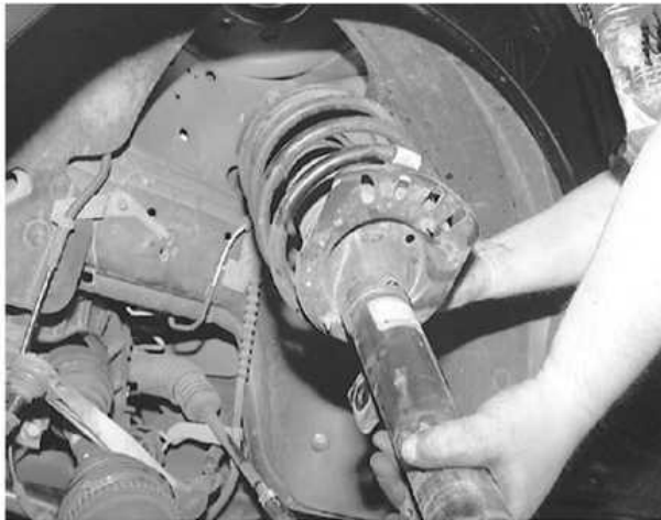
Remove the strut out the bottom to remove it from the vehicle
