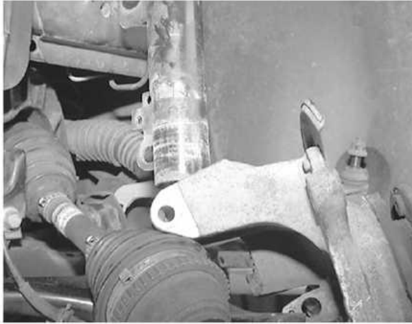
... remove the strut from the knuckle
