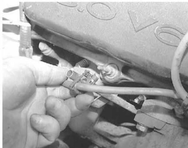
Remove the spark plug wire retainers from the valve cover retaining studs.
