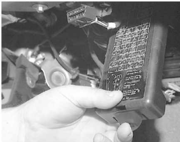
Remove the fuse panel cover
