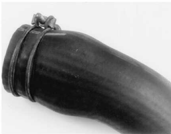
A soft spongy hose (identifiable by the swollen section) will eventually burst and should be replaced
