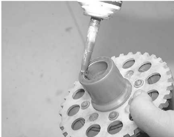
Apply a suitable sealant to the key-way of the crankshaft damper
