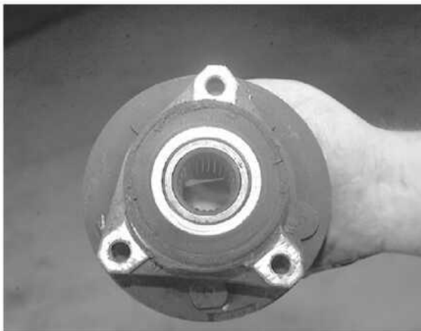
Inspect the bearings for damage and replace as necessary.
