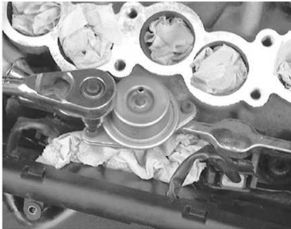
Remove the two pressure regulator retaining bolts and...
