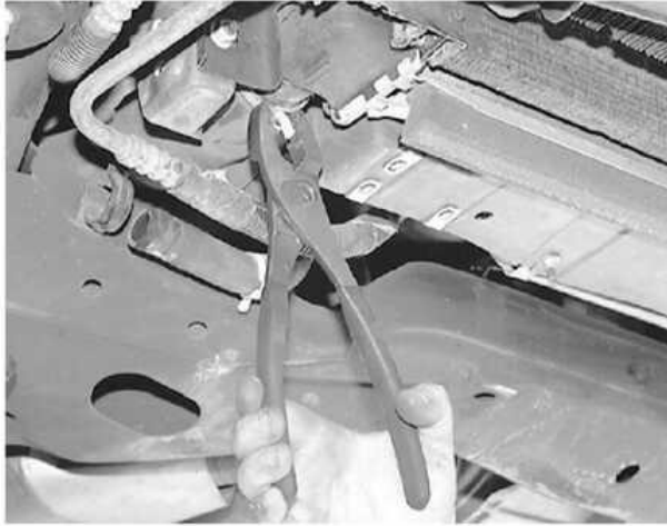
Remove the clamp from the lower radiator hose and...
