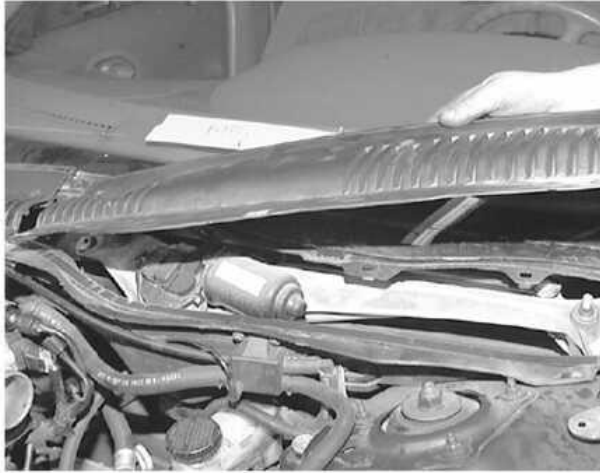
Carefully lift the cowl vent screen up and remove it from the vehicle.
