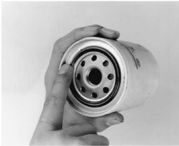
Before installing a new oil filter, lightly coat the rubber gasket with clean engine oil
