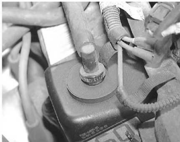
The PCV valve is located in the right hand (rear) valve cover-3.0L (OHV) engine
