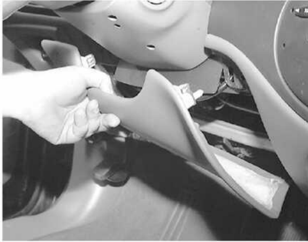
... remove the knee bolster panel from the vehicle
