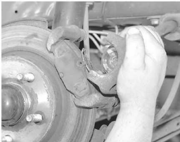
Carefully slide the caliper from the caliper bracket and off of the rotor
