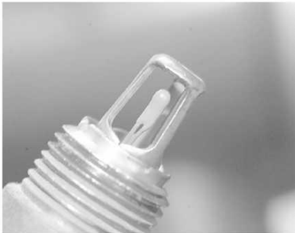
The tip of the IAT sensor has an exposed thermistor that changes the resistance of the sensor based upon the force of the air rushing past it
