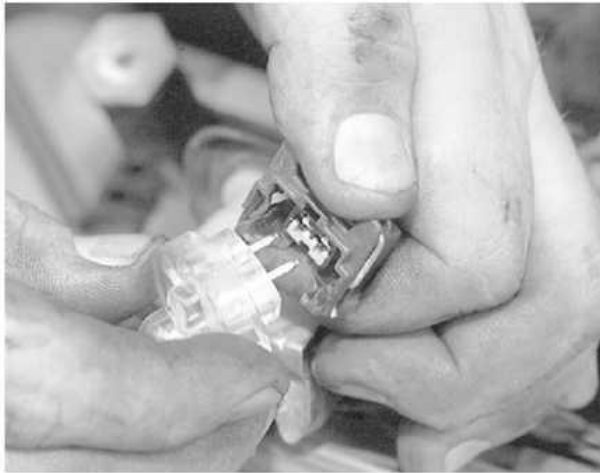
Plug the correct "noid" light directly into the injector harness connector.
