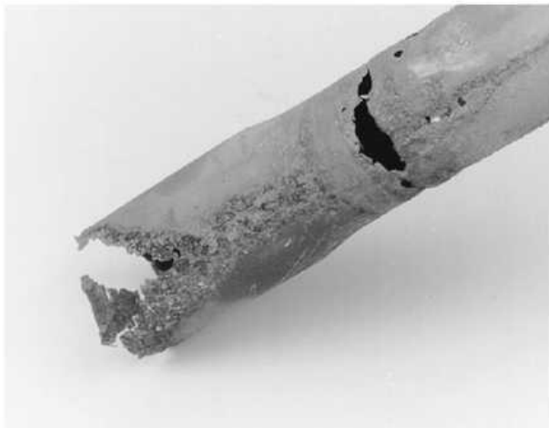
Example of a badly deteriorated exhaust pipe
