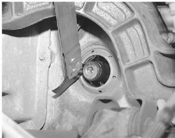
Using a suitable seal puller, remove the axle seal from the transaxle
