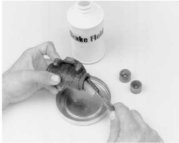
... and the bore of the wheel cylinder
