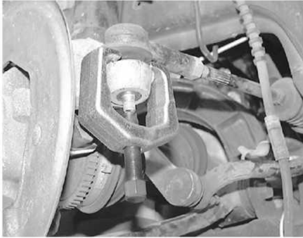
A special puller is recommended for removing the tie rod end from the knuckle.
