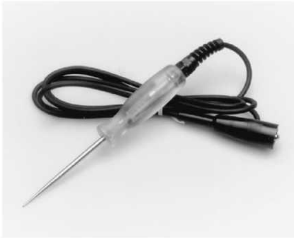
A 12 volt test light is used to detect the presence of voltage in a circuit
