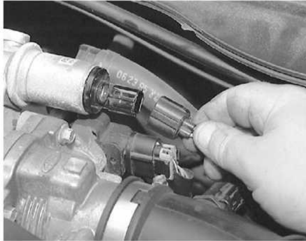
Detach the IAC valve connector.
