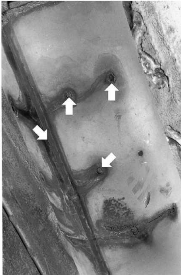
Check the muffler for rotted spot welds and seams
