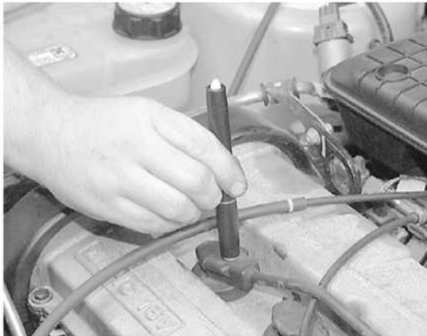
This spark tester is the easiest to use - just place it on a plug wire and the spark voltage is detected and the bulb on the top will flash with each pulse
