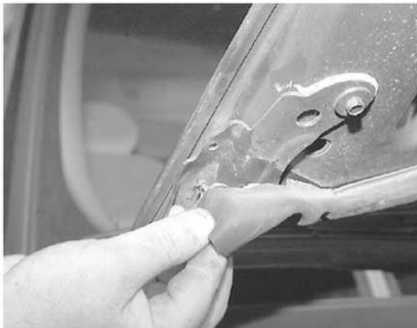
Peel back the weatherstripping protecting the bottom of the hood-to-cowl junction point, so that it clears the hood hinges
