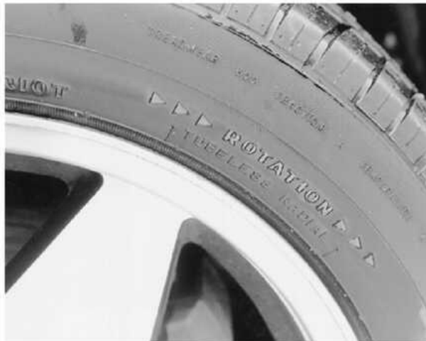
Unidirectional tires are identifiable by sidewall arrows and/or the word "rotation"
