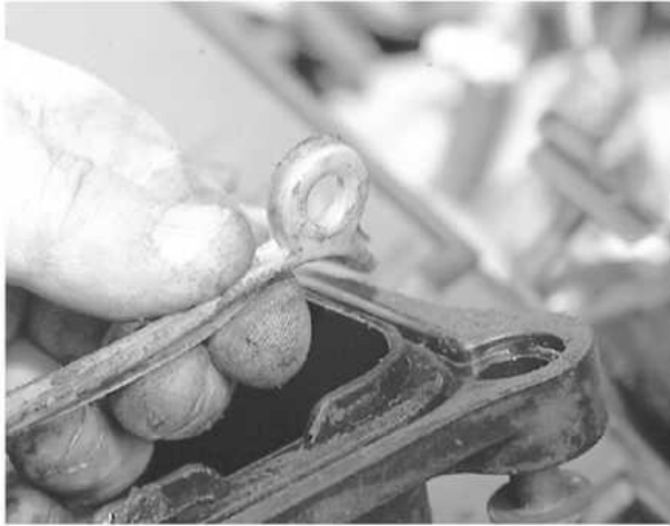
Remove the valve cover gasket from the valve cover
