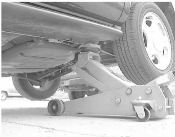
Place the jack under the body seam to lift the rear of the vehicle
