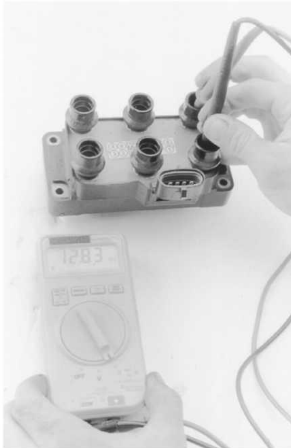
Testing the coil secondary resistance between the ignition wire terminals
