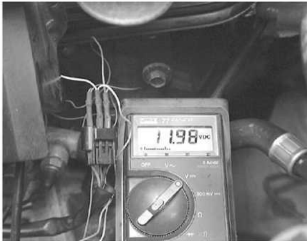
Testing the VPWR circuit of the CMP sensor
