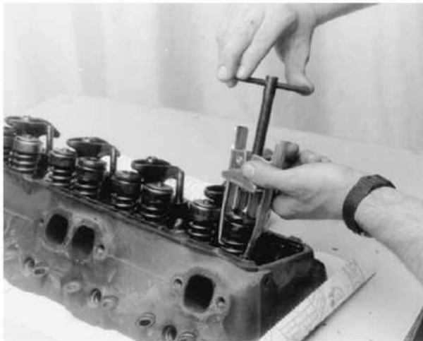
When removing an OHV valve spring, use a compressor tool to relieve the tension from the retainer
