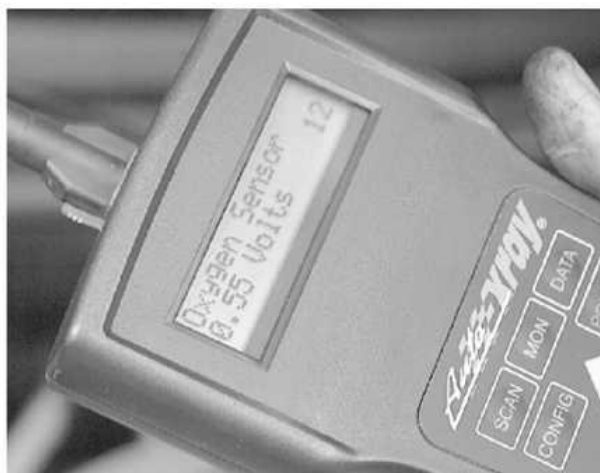
The voltage of the HO 2 S should be between 0.1 and 1.0 volts DC with the engine running.
