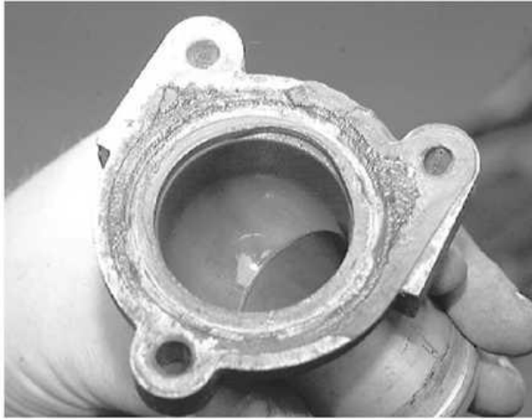
Inspect the water outlet connection for cracks or damage
