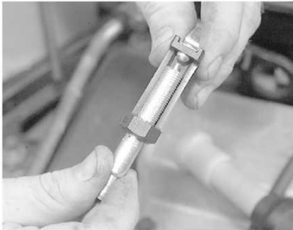
This spark tester has an adjustable air gap for measuring spark strength and testing different voltage ignition systems
