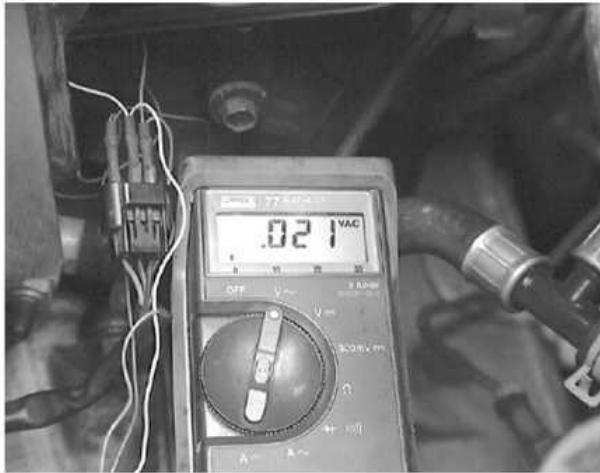
Testing the CMP sensor for voltage as the engine is running
