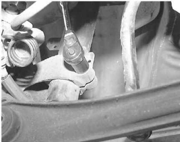
Remove the strut-to-spindle attaching bolt and...
