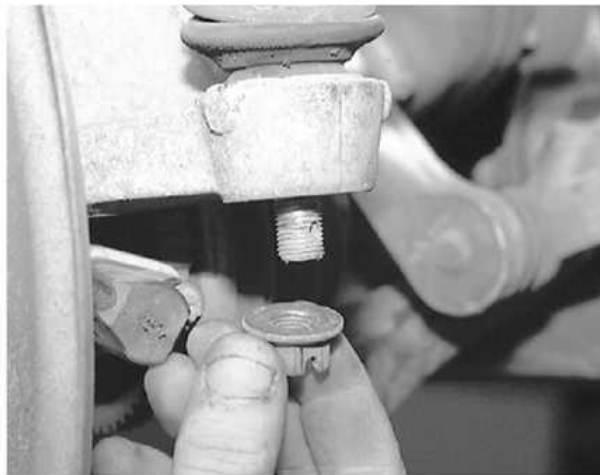
... remove the retaining nut from the tie rod end
