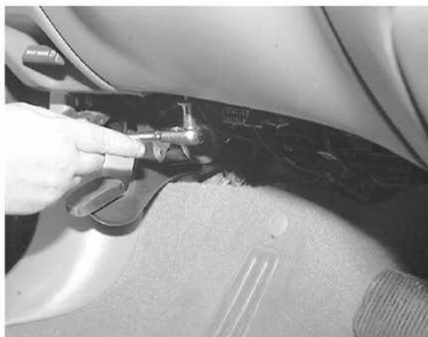
Remove the knee bolster panel retaining screws and...
