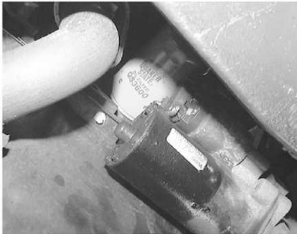
The oil filter is located on the engine, just above the starter-3.0L OHV
