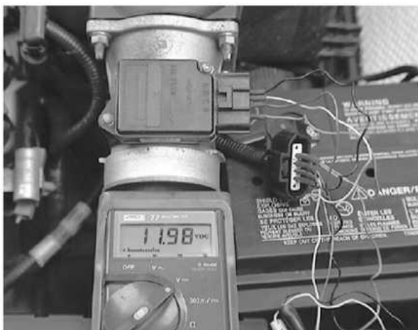
Testing the VPWR circuit of the MAF sensor
