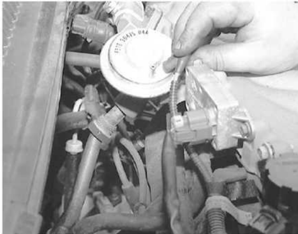
Tag and disconnect the EGR vacuum hose
