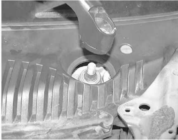
... remove the arm from the pivot
