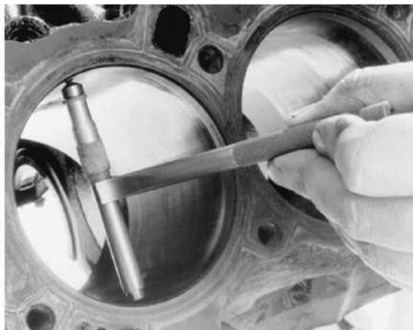
Use a telescoping gauge to measure the cylinder bore diameter—take several readings within the same bore
