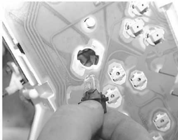
Rotate the sockets to remove the instrument cluster socket and bulb assembly
