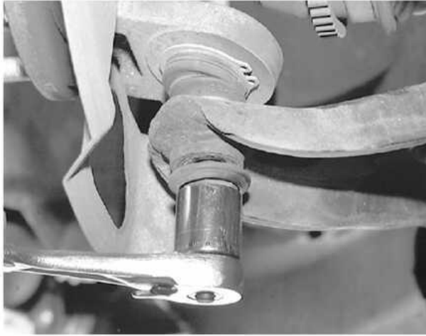
Loosen the ball joint nut and...
