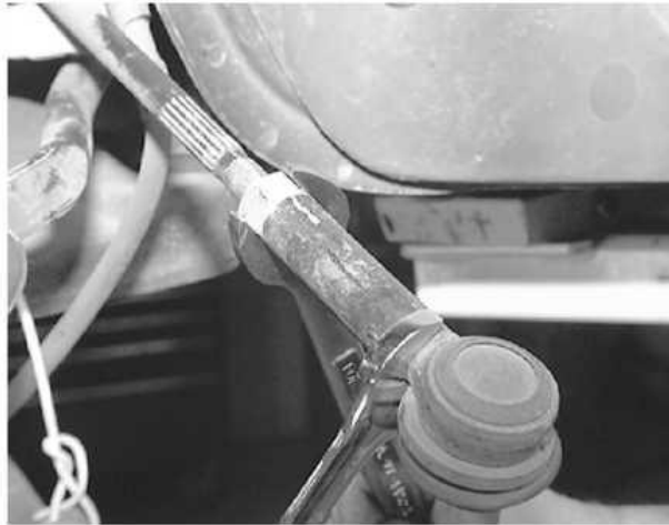
Use two wrenches, one to hold the inner tie rod, and one to loosen the jam nut
