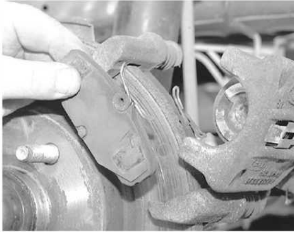
Remove the brake pads from the caliper bracket
