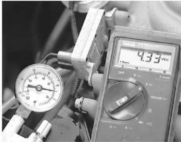
Apply vacuum to the DPFE and verify the signal return voltage is greater than 4.0 volts D/C
