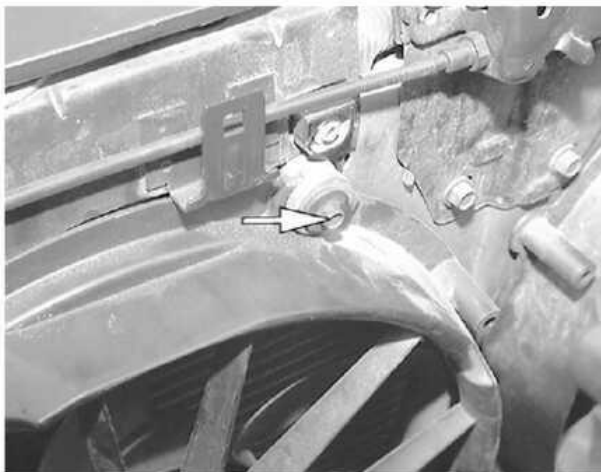
Remove the fan retaining bolts and...
