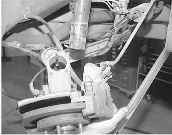
... separate the strut from the spindle
