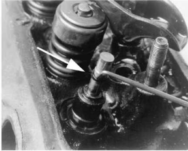
Remove the valve seal from the valve stem-O-ring type seal shown
