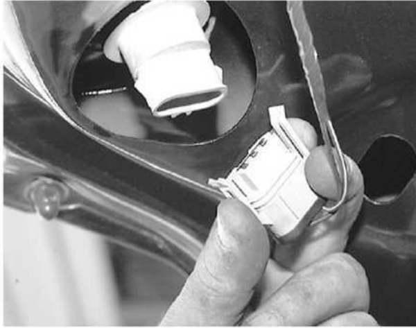
Detach the connector for the back-up lamp bulbs
