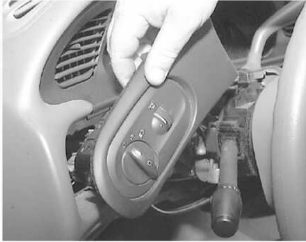
Carefully pry the headlight switch and finish panel away from the instrument panel
