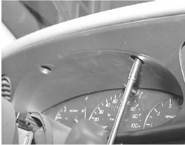
Remove the cluster finish panel upper retaining screws and...
