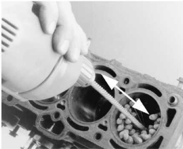
Use a ball type cylinder hone to remove any glaze and provide a new surface for seating the piston rings
