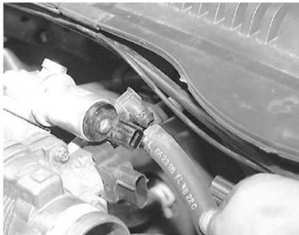
Tag and disconnect the booster vacuum hose from the vacuum fitting on the upper intake manifold
