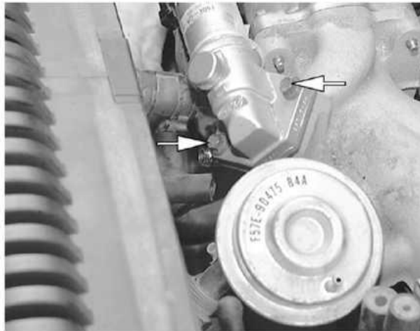
The IAC valve is retained by two bolts.
