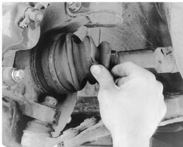
CV-boots must be inspected periodically for damage
