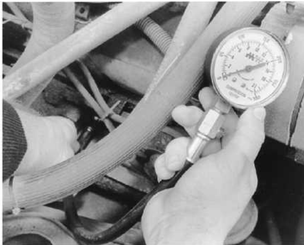
A screw-in type compression gauge is recommended for compression testing
