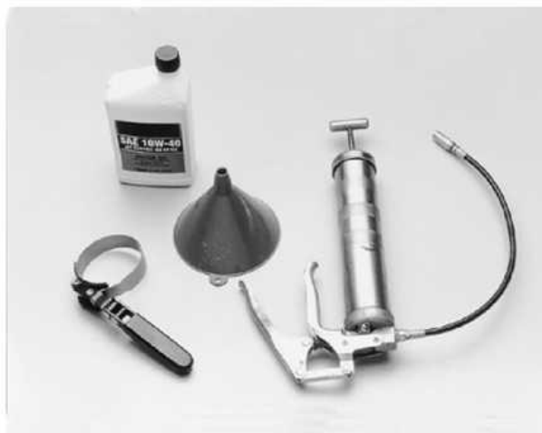
A few inexpensive lubrication tools will make maintenance easier
