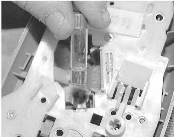
Pull the bulb straight out to remove it from the socket
