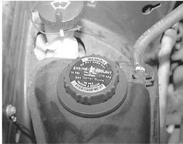
Remove the cap from the coolant recovery tank
