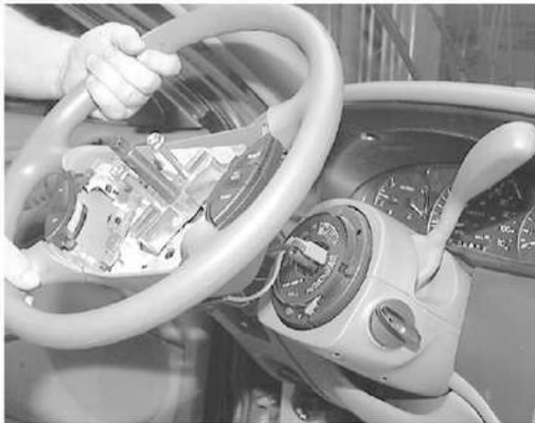
... remove the steering wheel
