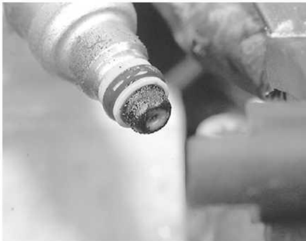
Inspect the injector tip for deposits and dirt build-up and replace if necessary
