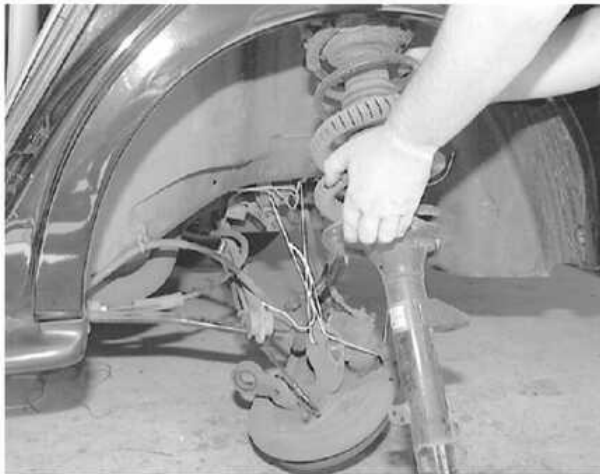
Remove the strut from the vehicle
