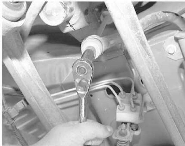
Remove the sway bar link-to-sway bar nuts
