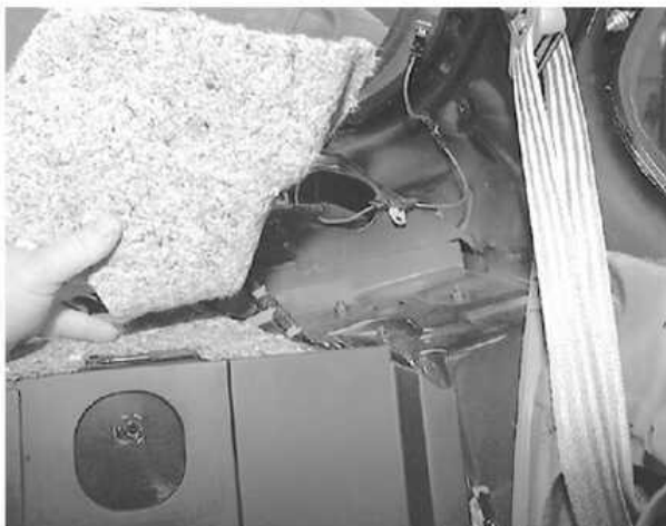
Remove the trim to access the strut upper mounting bolts
