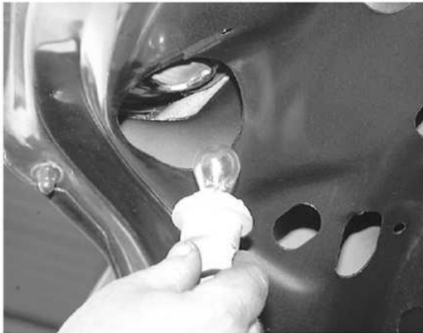
Rotate the bulb socket from the lens
