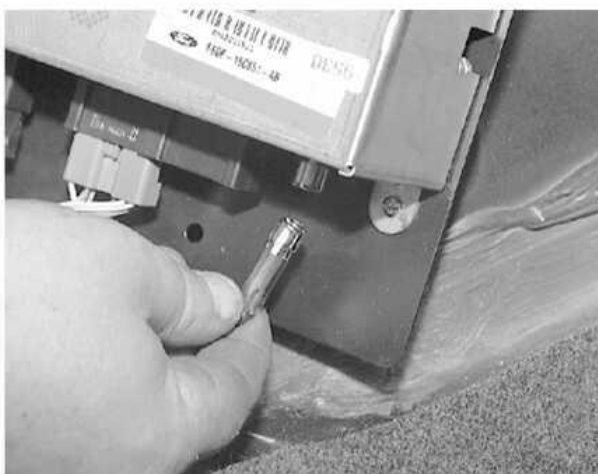
Disconnect the antenna from the rear chassis unit
