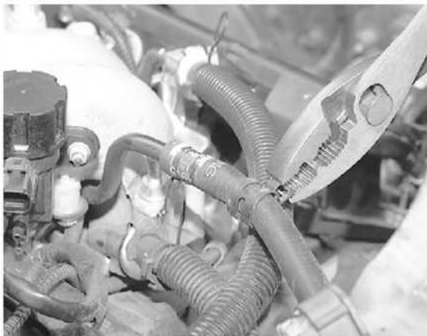
Remove the throttle body coolant hose clamp and...
