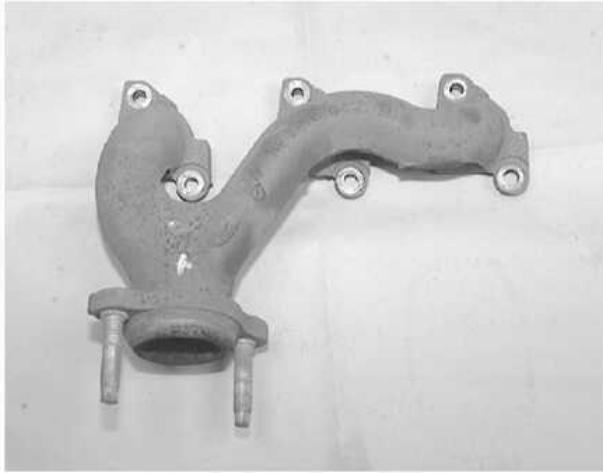
The exhaust manifold-removed from the vehicle
