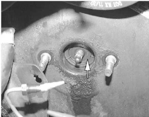
Replace the groove seal in the booster assembly before installing the new master cylinder
