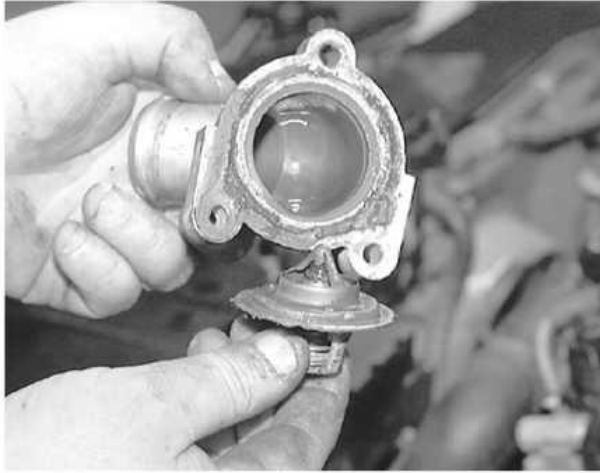
Remove the thermostat from the water outlet
