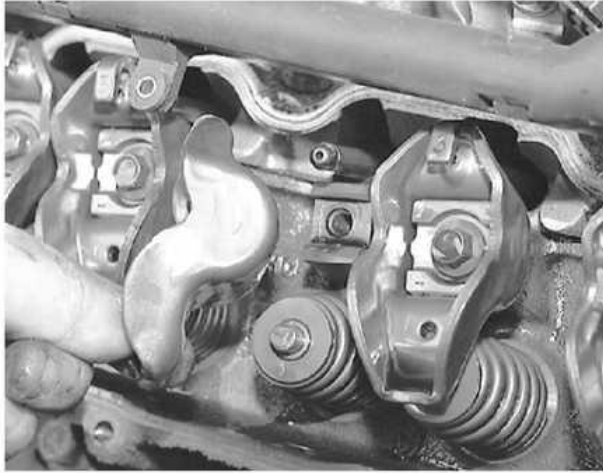
Lift the rocker arm off of the cylinder head and remove it from the engine
