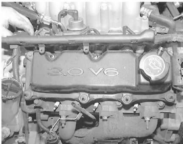
... remove the harness from the valve cover retaining studs
