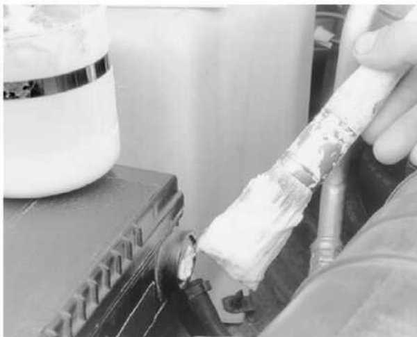
The battery terminal can also be cleaned using a solution of baking soda and water
