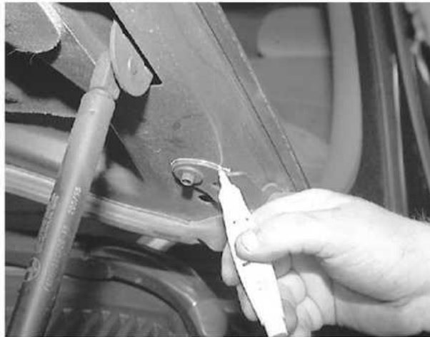
Matchmark the hood hinge location on the hood
