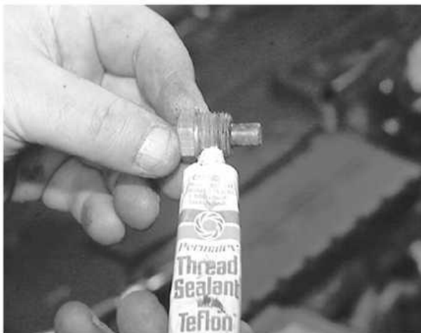
Before installing the temperature gauge sending, coat the threads with a suitable thread sealant
