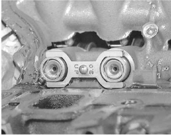
The lifters are held by a retainer
