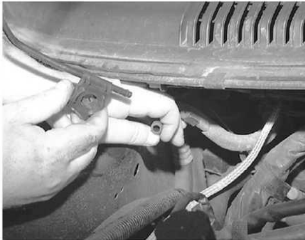
Disconnect the washer fluid hoses
