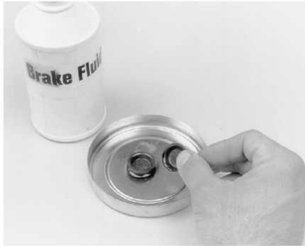
Lubricate the cup seals with brake fluid
