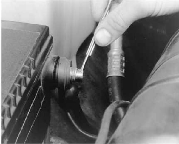
Loosen the battery cable retaining nut...
