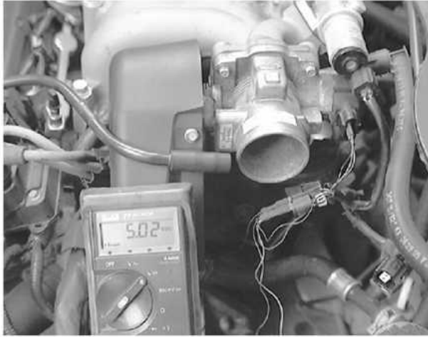
Testing the SIG circuit to the TP sensor
