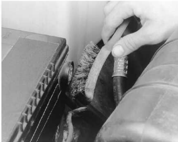
The wire brush can also be used to remove any corrosion or dirt from the battery terminal
