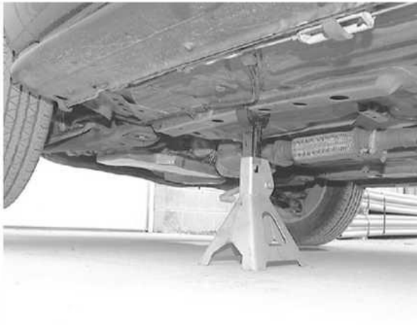
Also place the jack stand under the frame rails to support the front of the vehicle
