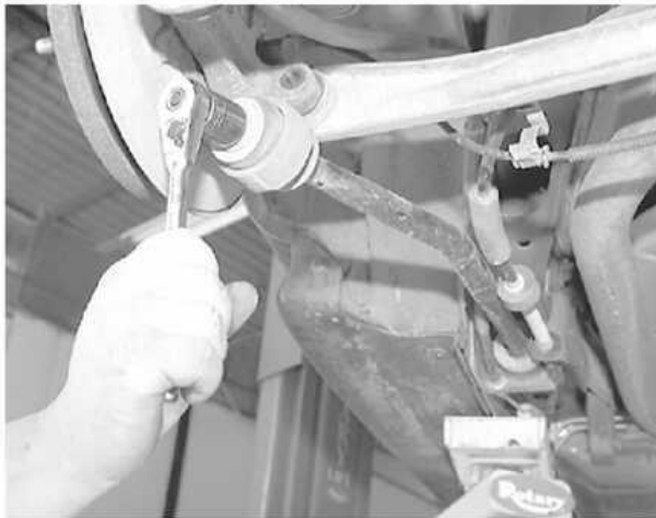
Loosen the tension strut-to-spindle retaining bolt and remove the tension strut from the spindle
