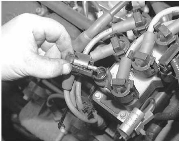
Squeeze the retaining tabs to remove the plug wires from the coil pack
