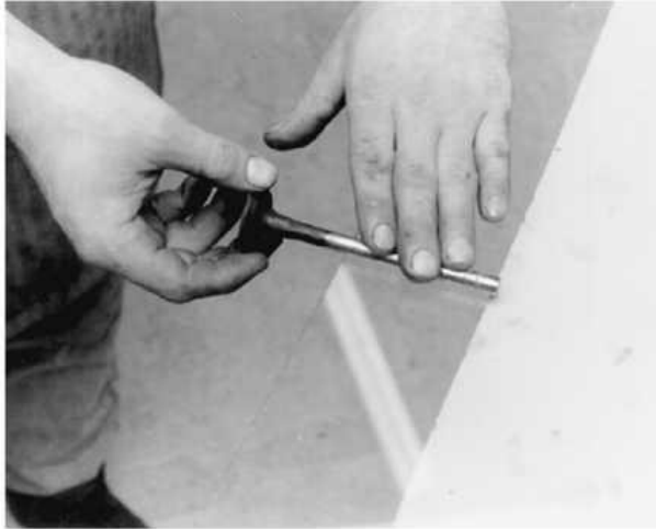
Valve stems may be rolled on a flat surface to check for bends
