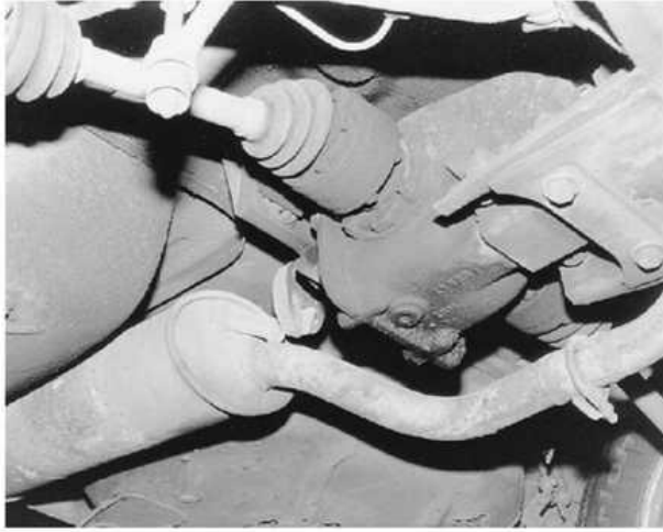
Make sure the exhaust components are not contacting the body or suspension
