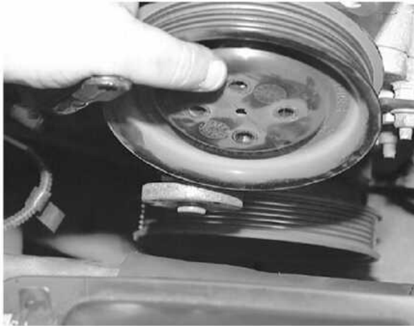
Remove the pulley from the water pump
