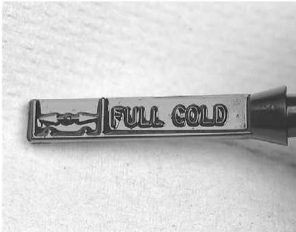
The power steering fluid level dipstick has a FULL COLD side and ...
