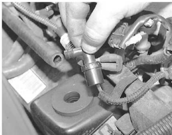
Remove the PCV valve from the valve cover grommet and ventilation hose | 3.0L (OHV) engine
