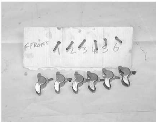
Be sure to number and separate the rocker arms and pushrods for installation
