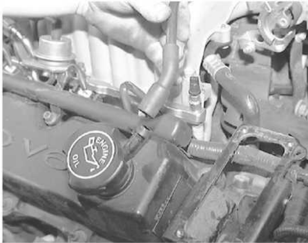
Remove the oil separator hose from the oil fill cap opening (LH valve cover only)
