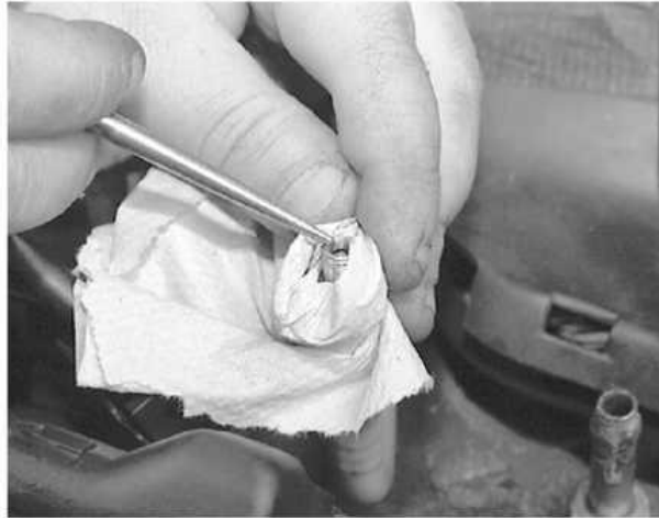
Depressing the pressure relief valve is one method to relieve the fuel pressure
