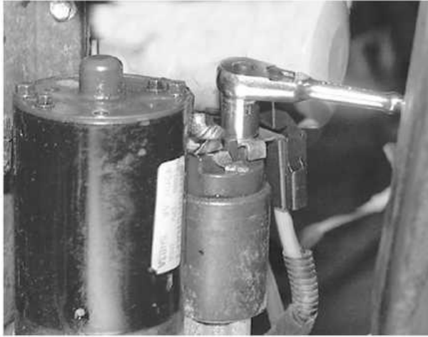
Remove the nut retaining the battery cable and...
