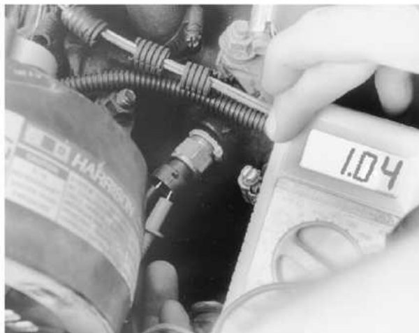
Checking the resistance of a coolant temperature sensor with an ohmmeter. Reading is 1.04 kilo ohms (1040 ohms)
