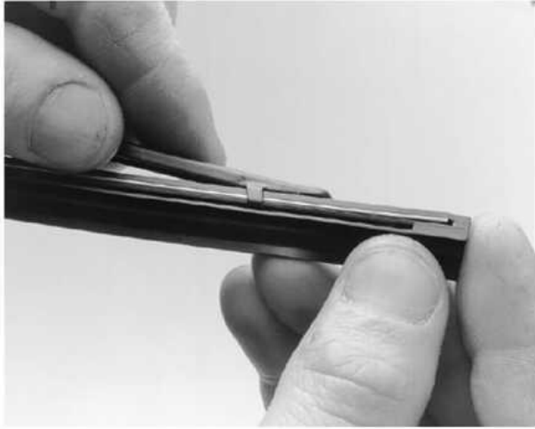
To remove and install a Lexor® wiper blade refill, slip out the old insert and slide in a new one.
