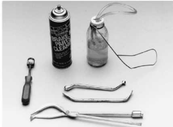
Although not always necessary, using specialized brake tools will save time
