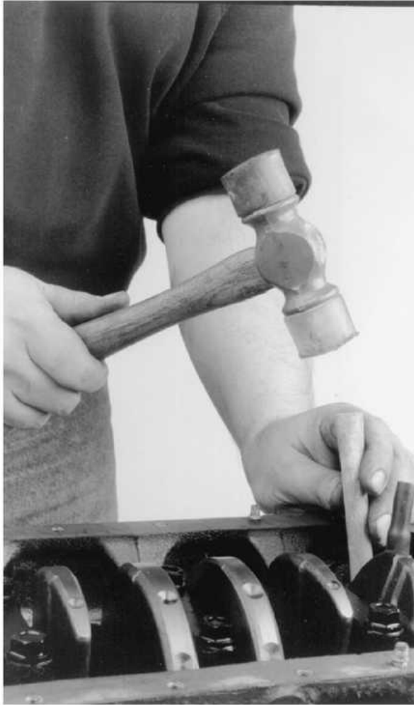
Carefully tap the piston out of the bore using a wooden dowel.
