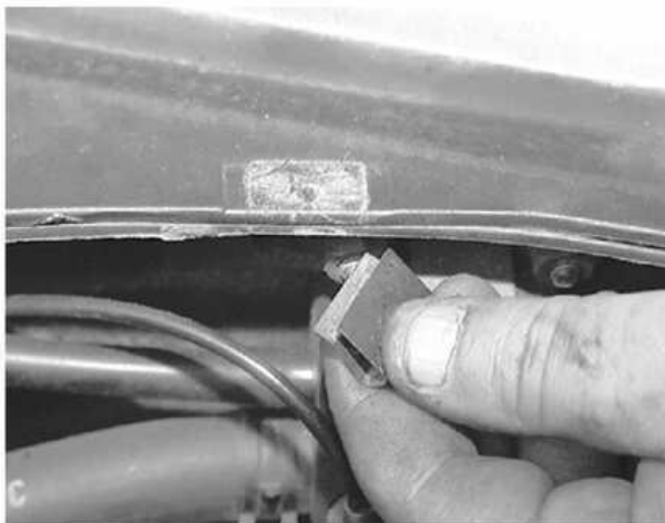
... screen-to-inner panel retaining clips from the cowl vent screens
