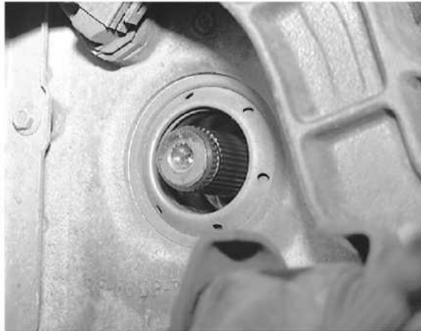
The axle seal is easily accessed once the halfshaft is removed
