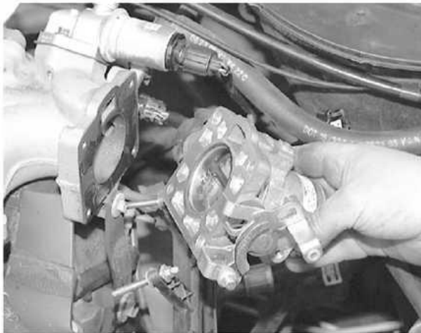
... remove the throttle body from the engine
