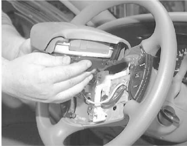
Carefully remove the air bag from the steering wheel to access the wiring connectors
