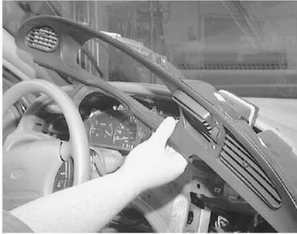
... remove the cluster finish panel from the vehicle
