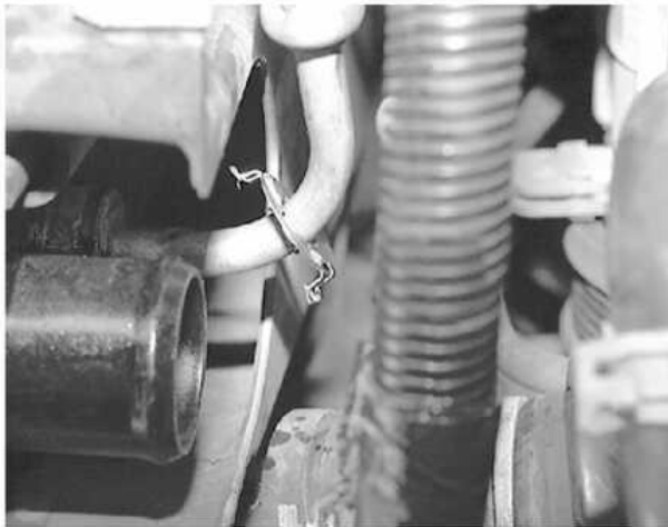
Remove the transmission cooler line retaining clips
