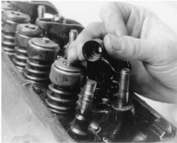
Removing an umbrella/positive type seal
