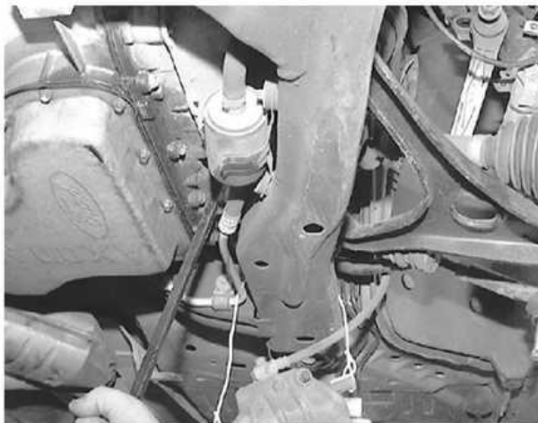
Using a pry bar or other suitable device, release the halfshaft from the transaxle and...
