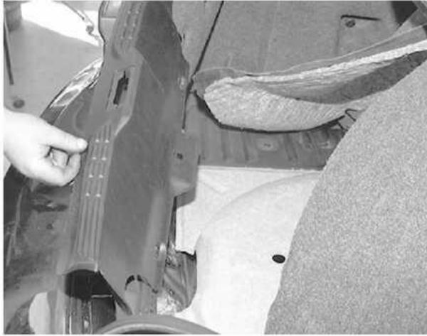
Remove the trim from the trunk
