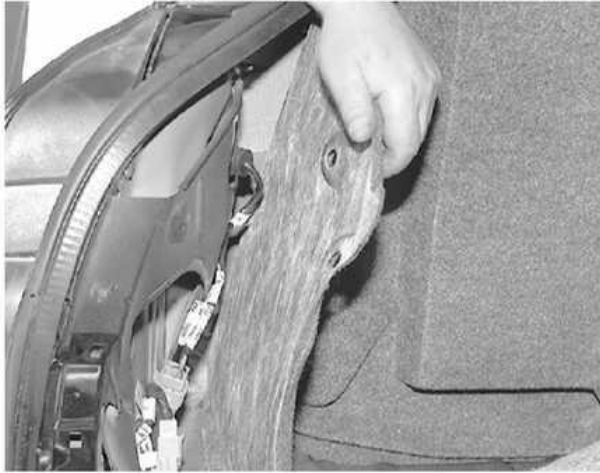
Carefully pull back the trim to access the taillamp retaining nuts. Remove the retaining nuts and...
