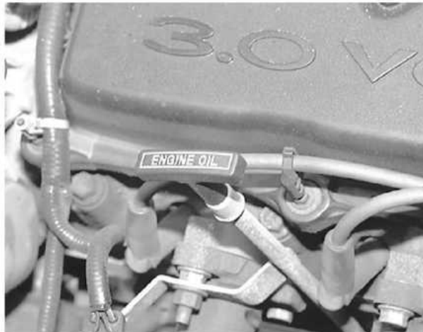
The oil level dipstick is located in front of the left-hand valve cover directly behind the radiator.
