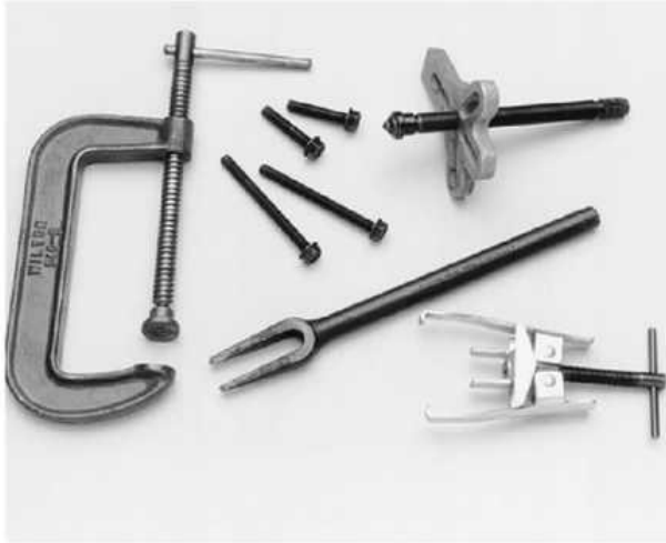
Various pullers, clamps and separator tools are needed for many larger, more complicated repairs
