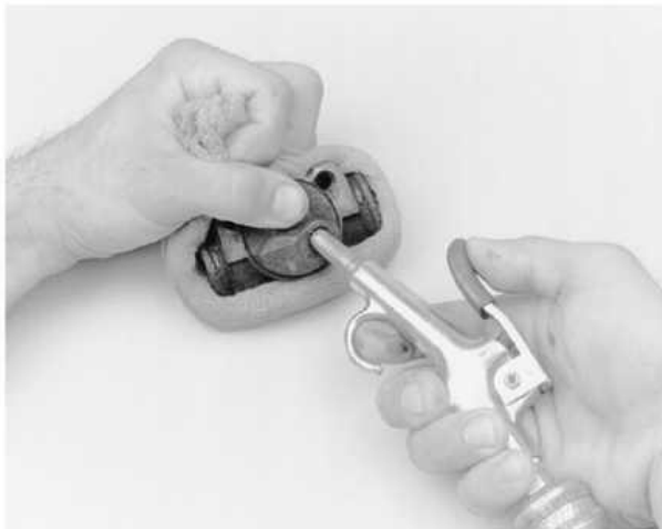
Compressed air can be used to remove the pistons and seals
