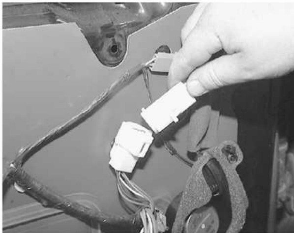
Detach the connector for the mirror
