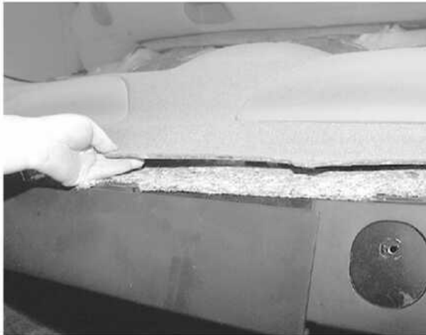
Remove the package shelf trim panel from the vehicle
