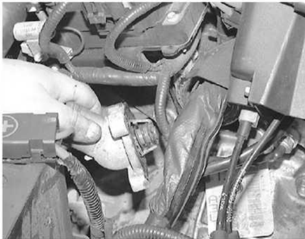
... remove the outlet from the engine
