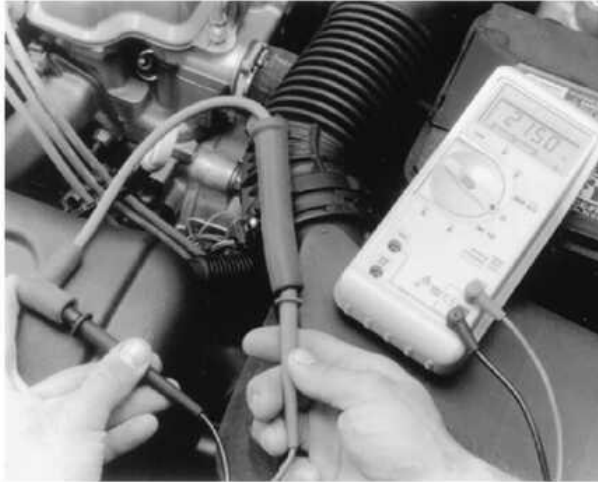
Checking individual plug wire resistance with a digital ohmmeter
