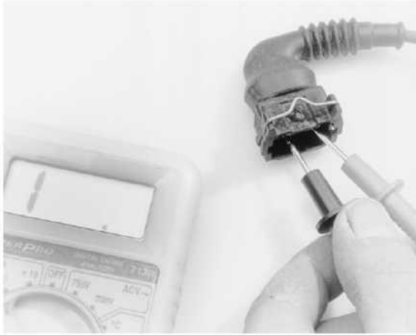
The infinite reading on this multimeter indicates that the circuit is open
