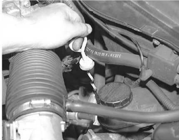
Remove the transaxle dipstick from the tube
