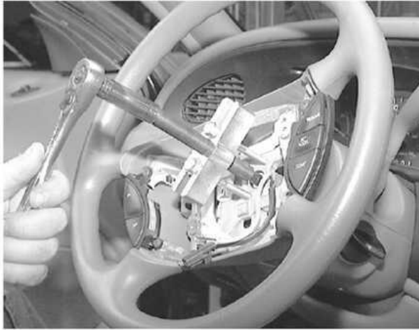
Install a suitable puller and tighten the forcing screw to...
