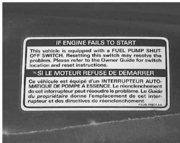
This label is usually attached to the underside of the hood. It is a reminder that the inertia switch could have been opened if the vehicle was involved in an accident.
