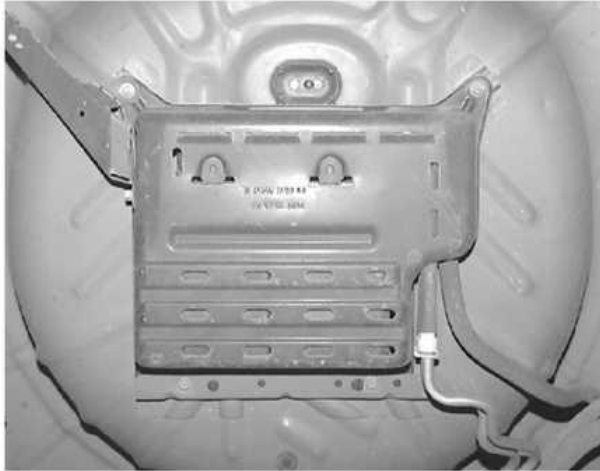
Location of evaporative emission canister and its related components - 3.0L (OHV) non-flexible-fuel, 3.0L (DOHC) and 3.4L (DOHC) vehicles
