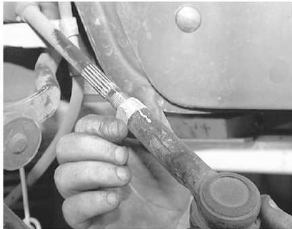
Back the jam nut off ONE TURN ONLY and then unthread the tie rod end from the inner tie rod and...
