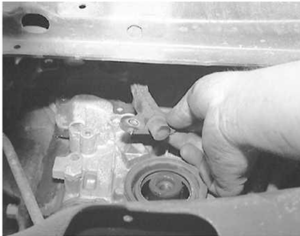
... remove the CKP sensor from the engine
