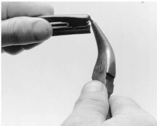
On Trico® wiper blades, the tab at the end of the blade must be turned up...
