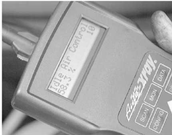
The IAC can be monitored with an appropriate and Data-stream capable scan tool
