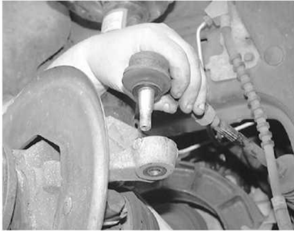
Remove the tie rod end from the steering knuckle.
