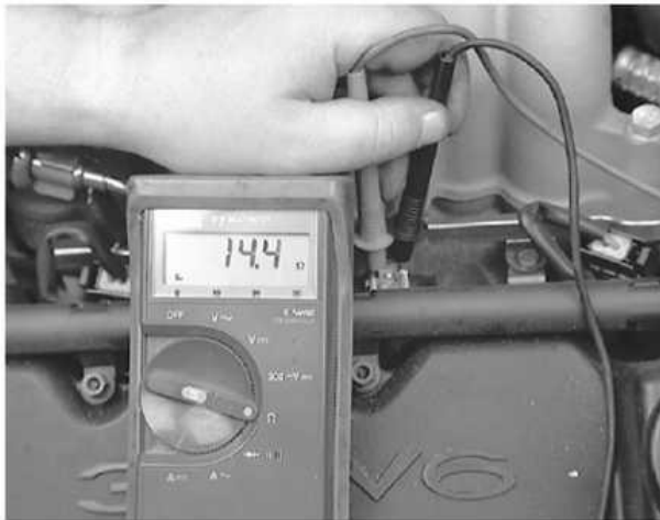
Probe the two terminals of a fuel injector to check its resistance
