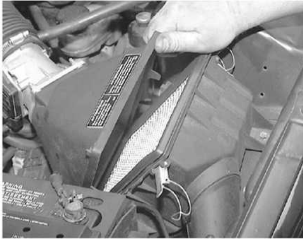
... lift the air cleaner housing cover to access the filter element
