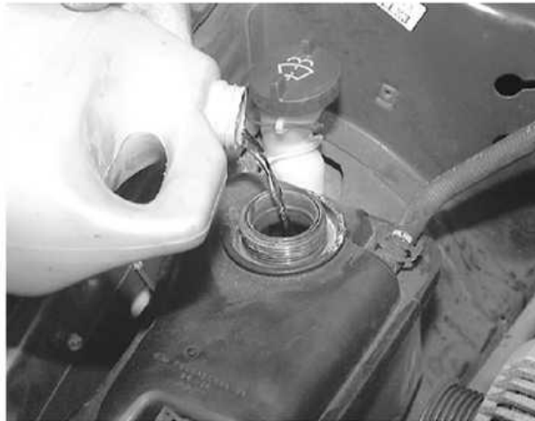
Pour the proper 50/50 coolant-to-water ratio directly into the coolant recovery tank
