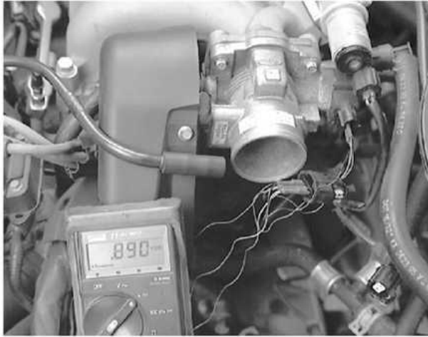
Testing the SIG RTN circuit of the TP sensor
