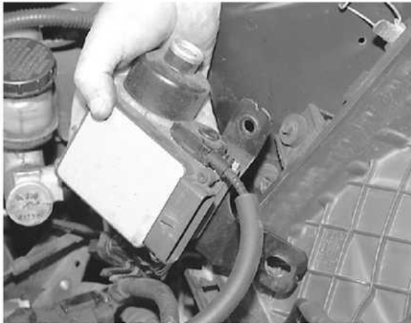
Remove the actuator retaining nuts and position the actuator out of the way
