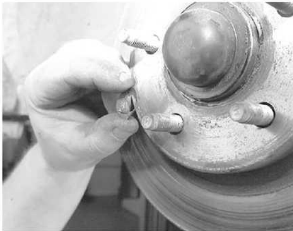
... retainer nuts placed on the rotors from the assembly line
