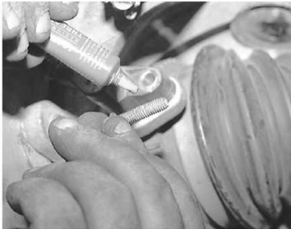
Apply a quality thread locking compound to the retaining bolt before installation
