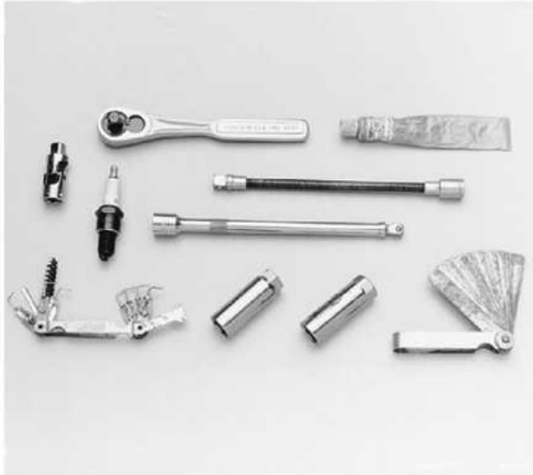
A variety of tools and gauges should be used for spark plug gapping and installation
