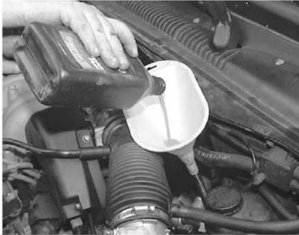
Place a funnel into the transaxle dipstick tube and add the fluid as necessary
