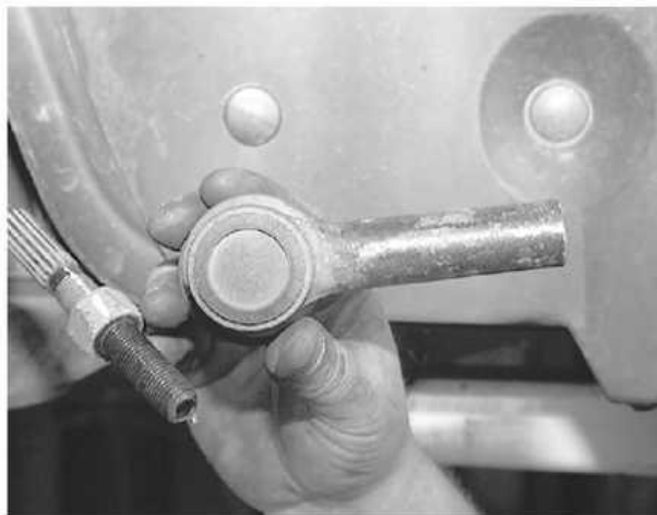
... remove the tie rod end from the inner tie rod.
