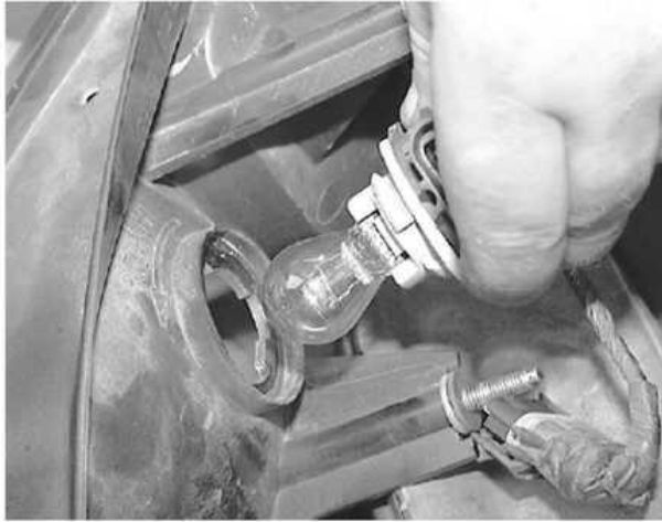
... rotate the bulb sockets from the taillamp assembly
