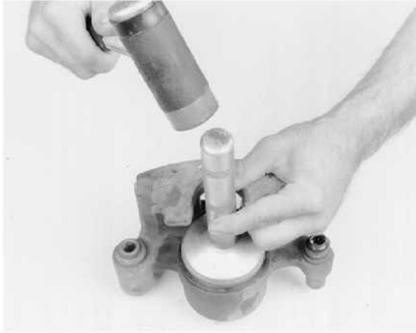
Use the proper size driving tool and a mallet to properly seal the boots in the caliper housing
