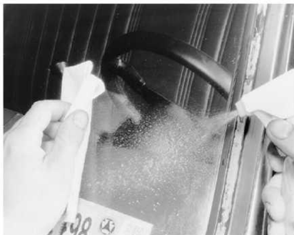
To repair a chip, clean the windshield with glass cleaner and dry it completely.
