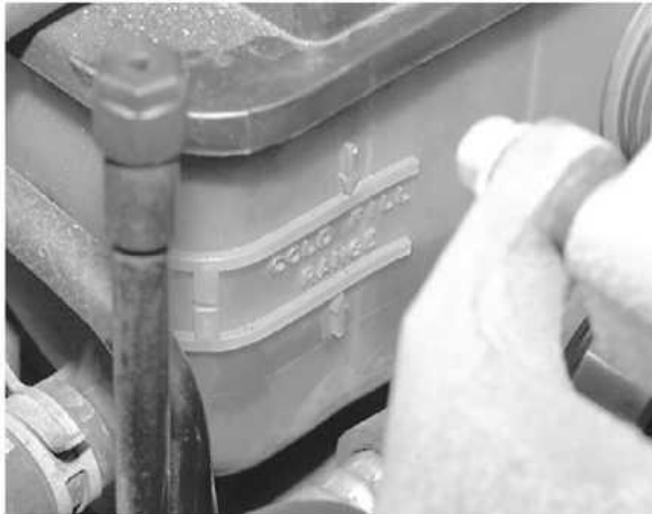
The coolant level should be between the COLD FILL levels on the coolant recovery tank.
