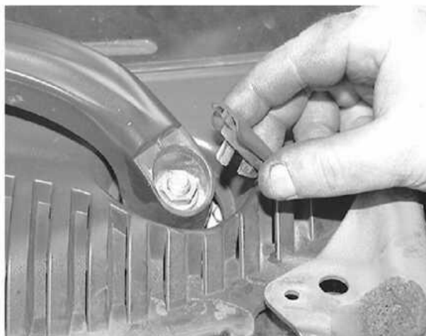
Remove the wiper arm retaining nut cover
