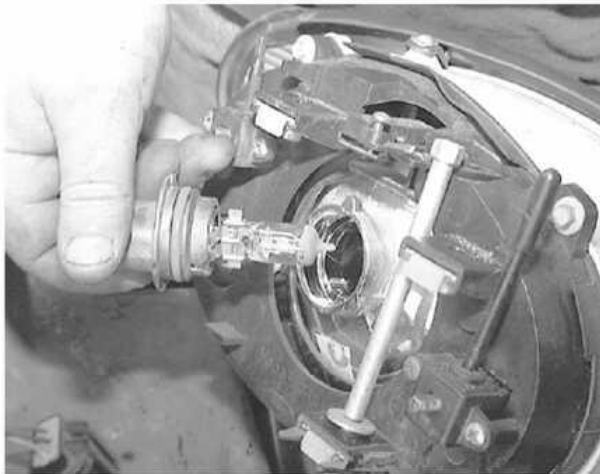
... remove the headlight bulb from the lens assembly
