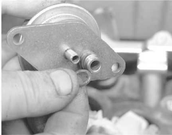
Replace the O-rings on the pressure regulator and...
