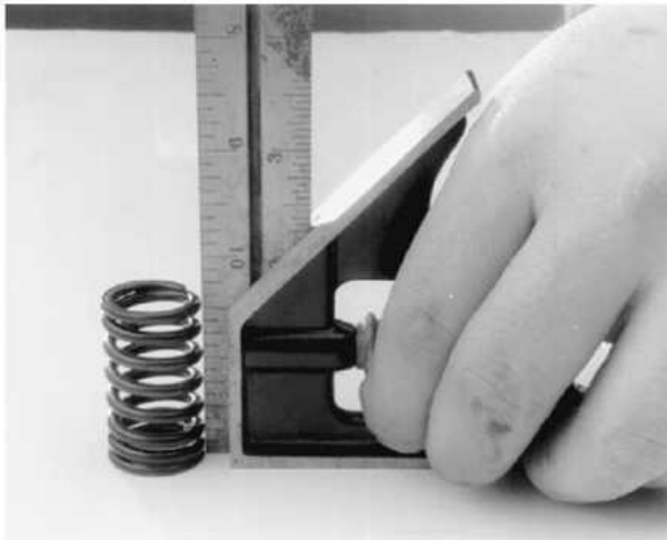
Check the valve spring for squareness on a flat surface; a carpenter's square can be used
